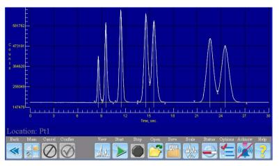
MOCON's PetroAlert® analyzers have been used by surface loggers for more than 40 years to provide qualitative and quantitative hydrocarbon measurements. The PetroAlert 9100 GC provides C1-C5 concentrations in less than 30 seconds using a flame ionization detector, with options to add additional compounds such as alkenes.
