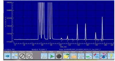
This is an example of one of the many custom applications we have developed for the oil & gas exploration industry. This application reported all C6, C7, and C8 hydrocarbons and their isomers as a total per carbon number, and isolated and quantified selected aromatic hydrocarbons. Other custom applications have been C1-C10 (as totals), C6-C10, and C1-C5 with BTEX.
