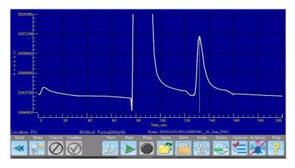
The Baseline 9100 provides low level measurement of formaldehyde in ambient air. This instrument is commonly utilized in industrial facilities and paint booths to monitor workplace exposure limits. The sample is first separated into individual components, then sent to a methanizer where formaldehyde is converted to methane then detected and quantified by the FID.
