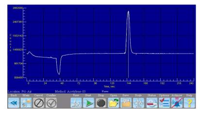
Baseline 9100 GCs are specifically applicated to monitor low part-perbillion levels of toxic gases, at dozens of sample points with multi-level alarms, and provide daily TWA reports for each location. Depending upon the specific industry requirement, the Baseline 9100 can be customized by MOCON to detect many different toxic gases well below OSHA action levels while avoiding the potential false positive alarms that are common with total gas detectors.
